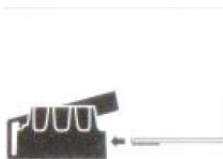
Figure 6.0 – Place the test strip in the cap with the pad covering the small opening on the cap.
